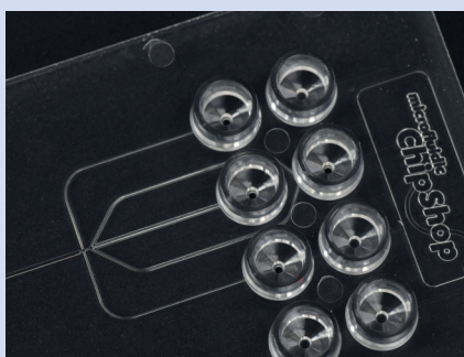
Detailed inlet and channel design of Fluidic 163
