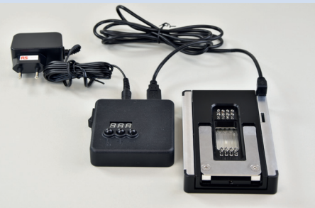
The complete setup of a LOC CCI 1 with heating elements. In contrast, the LOC HP does not include temperature control units.
