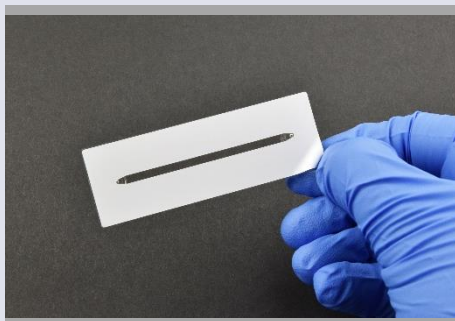
Peel off the protective film of the double-sided tape starting from one corner
