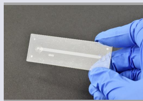
Check for remaining air inclusions by holding the chip against the light
