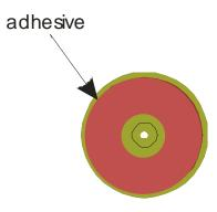
3. Place the bonded port connector on the chip, being careful to align the connector so the shoulder sits inside the port and the bonded area is flush with the substrate.
