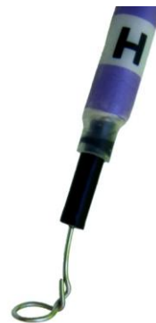
Figure 2. Platinum electrode inserted in LabSmith HVC high voltage cable termination.
