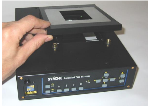
Removing the microscope stage
