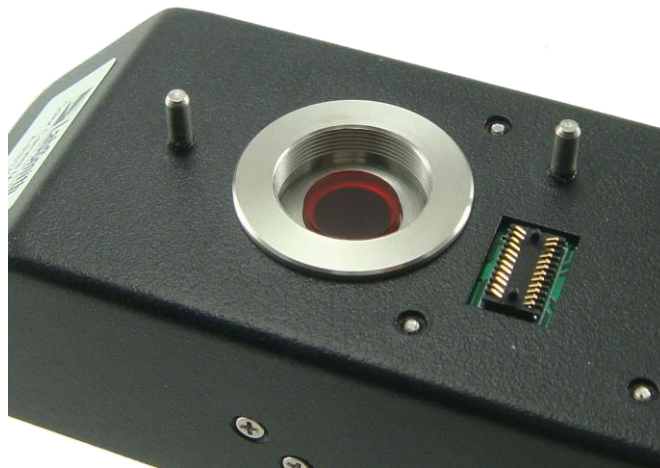
Filter installed in an optics module (foam washer is placed on top of filter)
