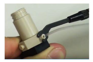
**CAUTION**: Do not over-tighten the fitting, which will break the CapTite.
