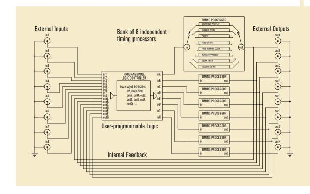
LC880 architecture: 8 inputs, timing channels, and outputs with trigger signal logic and routing.
