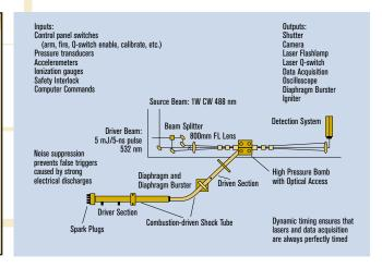
Trigger timing modes can be programmed via dialog controls. Logic is programmed using C-style syntax.
