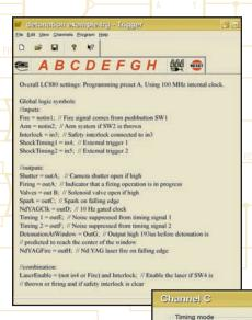
Programming in Trigger: Sample file in which an LC880 controls a camera shutter, two solenoid valves, a spark plug, and a Nd:YAG laser for a detonation experiment.
