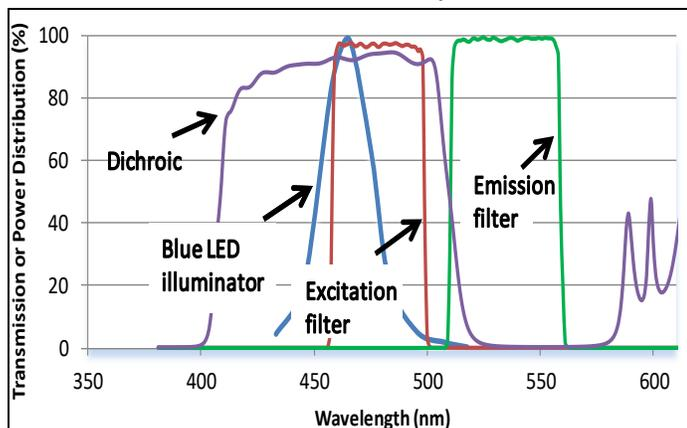
SVM340 EPI Spectral Specifications. Light transmitted vs. wavelength for light source and filters for EPI-BLUE module.
