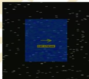
Image of a  $\mu$ PIV velocity probe of polystyrene beads in a microfluidic chip, moving under an applied electric field. Imaged using the SVM340 and LabSmith uScope software. Courtesy of Professor Blanca H. Lapizco-Encinas *et al*, Tecnológico de Monterrey (Monterrey, Mexico).
