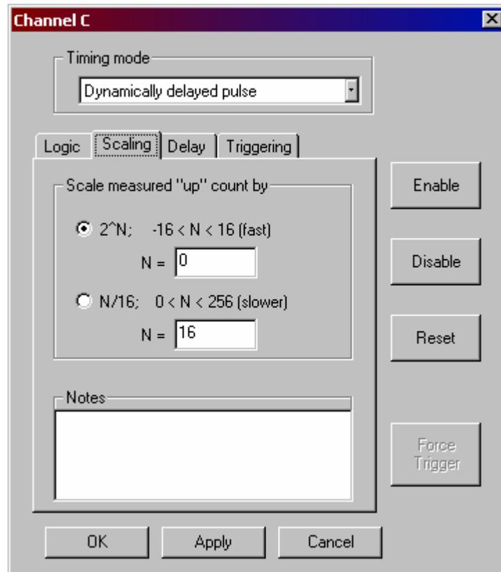
In the calculation of the delay, the measured delay between two pulses is scaled by a factor of  $2^N$ , where  $-16 < N < 16$ , or  $N/16$ , where  $0 < N < 256$ . The former scaling is faster and a scaling of 1:1 is fastest. Scaling can typically be done at rates  $> 50$  kHz.
